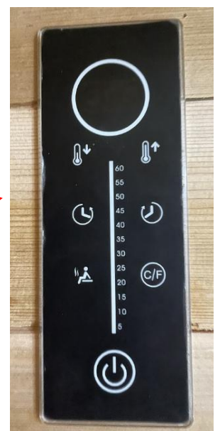
Sauna Control Panel has no Illumination
